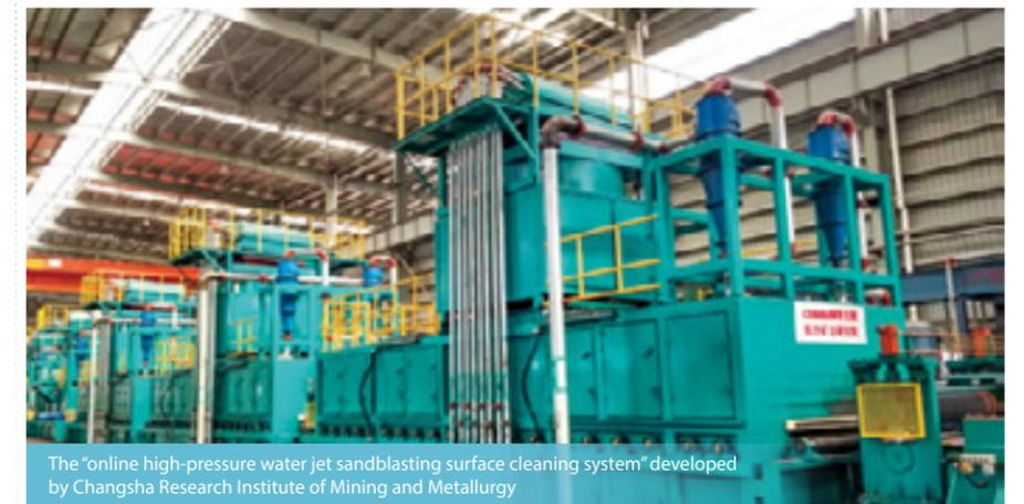
The “online high-pressure water jet sandblasting surface cleaning system” developed by Changsha Research Institute of Mining and Metallurgy
